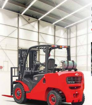
In developing the new XF Series, comfort and ease of operation is carefully considered, for example, to improve vibration levels, compound engine damper and full floating power train are adopted.
